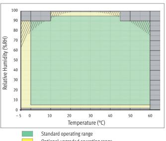
Optional upgraded operating range Condensation possible in chamber (dependent on ambient)
